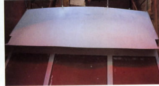
The steel is prepared for a topcoat of Awl Grip.
