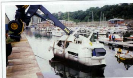
Above when a lift-out went wrong, the crane toppled over and impaled this Carver. The damage was extensive, but was 'invisibly mended' by GYS.
