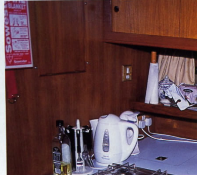
Above left opening this panel to trace the source of the smoke, fed the fire and caused an explosion. Above right the panel in the restored galley, minus the spice rack.
