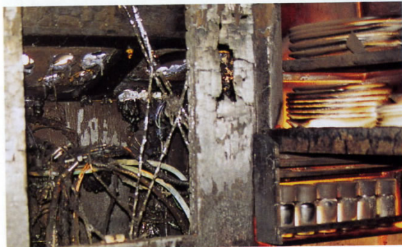
Above left opening this panel to trace the source of the smoke, fed the fire and caused an explosion. Above right the panel in the restored galley, minus the spice rack.
