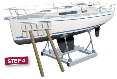
Put the mould in place and lay up from inside
