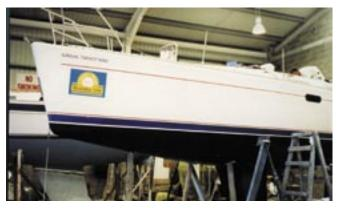
5 The finished job, complete with a fresh coat of antifouling, originalspec decals and a new toerail. From start to finish this job took about a month and cost £15,000.
