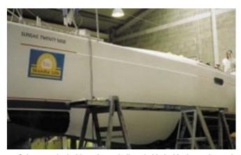
4 Colour-matched white gel coat, built up behind with chopped strand mat, has been used on the repair. Once the mould has been removed, additional layers of colour-matched gel coat will be applied from the outside. These will be repeatedly applied and sanded back until the whole hull is fair.
