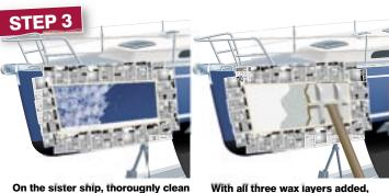
With all three wax layers added, you can now brush on two layers of gel coat, leaving each to cure to tackiness. The gel is then followed by some chopped strand mat, with foam or wood stiffeners bonded in for strength. Brace the whole thing so its weight won't allow it to fall
