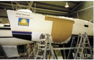
With the insides of the cut-marks tapered, sheets of Melamine hardboard are now used to recreate the hull shape. This is fairly quick, but will it be quite labour-intensive when it comes to flatting back the gel coat that has been laid up against it from the inside.
