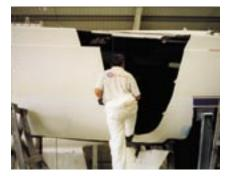
The first job is to cut away all the damage to beyond the last of the stress cracks. A fine soot is used to trace where the hairline cracks finally end. Note how all the antifouling has been stripped for some distance each side of the damage. To get to the hull, much of the internal furniture in this section had to be disassembled.
